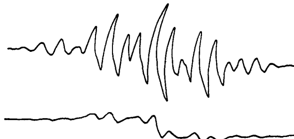
Fig. 2.—Spin resonance spectrum of 1.4 \times 10^{-3} M potassium naphthalenide in DME: above, no added naphthalene; below, naphthalene added at 0.218 M .
